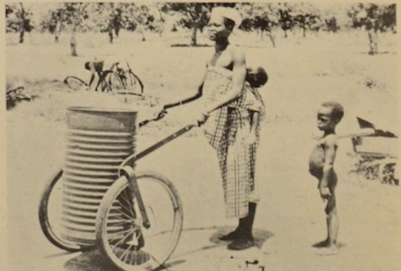
This piece of technology can carry enough water for one day. It can knock 48 woman-hours off the job of transporting water from a distant well to the village. It saves 200 miles of fetching and carrying and needs no fuel. It cost £1.
