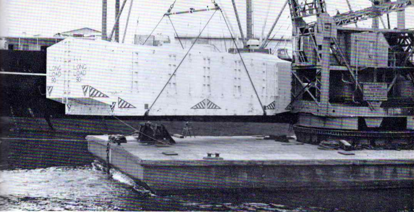
The Blue Streak being unloaded by floating crane.
