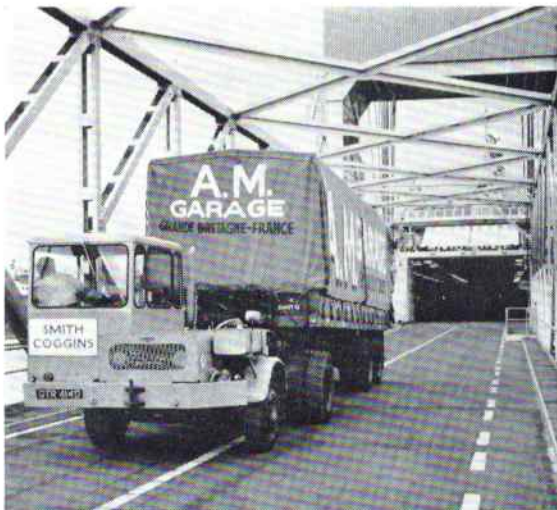
An articulated trailer being loaded into the main vehicle deck. Larger vehicles can be accommodated on the open deck above, which also has direct access by ramp-bridge.
