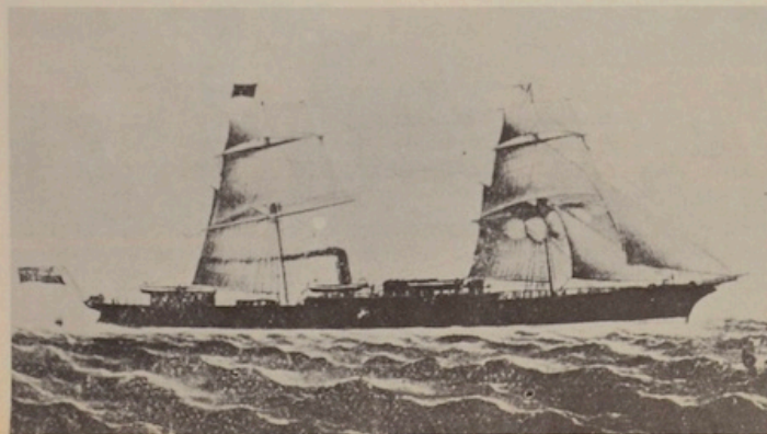
In 1874 the E & A Company placed orders with Glasgow shipyards for three modern design ships, far ahead of anything else on the Australian/Japan run at that time. Among them was the Brisbane, a 1503 ton steamer, fully rigged on both masts, easily distinguished by a large deckhouse amidships and aft. The Brisbane first sailed into Australian waters in February 1875. Brisbane had powerful compound engines of 250 nhp providing a service speed of 13 knots.
